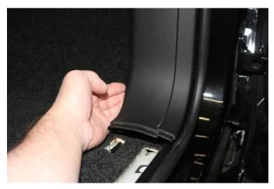
Remove the plastic panel, on the right side of the dash, by prying straight out:
