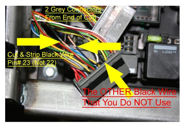
From the Smaller Grey Plug, crimp T-Taps onto **Both Red Wires and the Red/Blue Wire**, pay attention to which Red Wire is which when plugging in:
