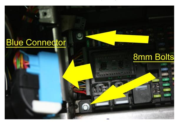
Reach up behind the CJB and remove 2 of the 3 plugs, Orange and Green. The Grey at the back is not needed. This is what the back of the CJB looks like:
