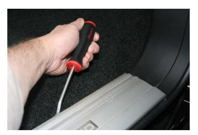
Pull towards the back of the vehicle and remove the passenger kick panel (no need to remove the red plugs that hold it in place, it will push back on to them):
